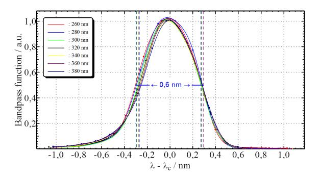
Bandpass function around centroid  $\lambda_c$  for different wavelengths with bandwidth (FWHM, dashed lines) indicated.
