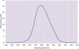
Bandpass filters can significantly reduce potential for stray light – akin to first half of a double monochromator
