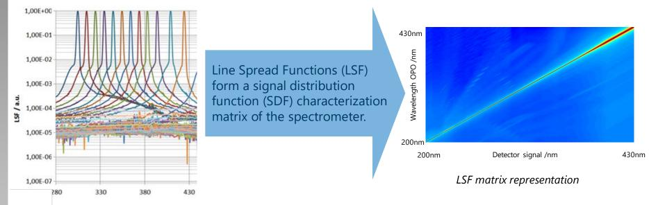
LSF of spectroradiometer measured using an OPO
