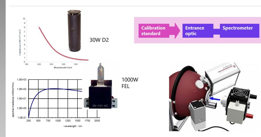
Tungsten halogen and deuterium lamps commonly used – but both have their limitations Calibration source needs to be suitable for required radiometric quantity and entrance optic
