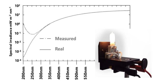
The amount of stray light in a measurement strongly depends on the light source and the spectrometer itself.
