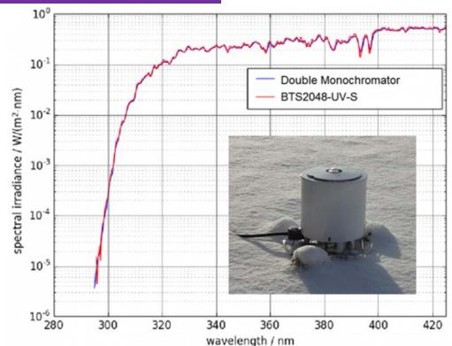
Comparison of a solar measurement with BTS2048-UV-S-WP and a double monochromator illustrates the high dynamic range of the stray light corrected array spectroradiometer
