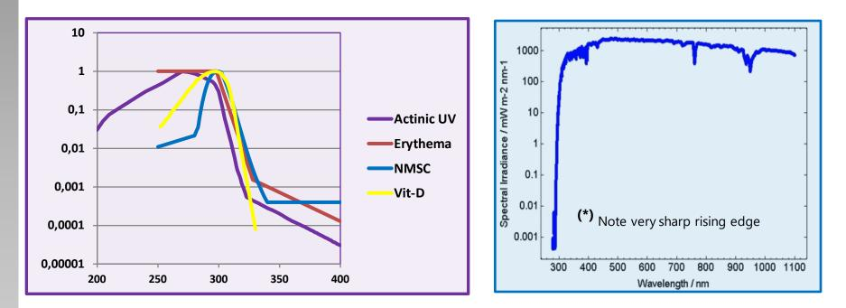
Calibration factors inversely proportional to responsivity Therefore, stray light component increasingly significant in deep UV
