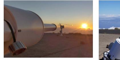
BTS2048-UV-S mounted on a solar tracker
