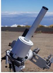
Ground-based spectroradiometer measurements of direct solar UV irradiance can be used to determine the Total Ozone Column (TOC) by applying the Beer-Lambert law in conjunction with the known absorption characteristics of ozone over the 290-350nm wavelength range. Suitable modelling is required to minimise the influences of other atmospheric attenuators [1].
